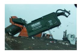
Several pieces of equipment (dump trucks, leaf vacuums, sanitation trucks, and sweepers) have lift gates or bodies that can be raised. Under normal operations, workers are not permitted to go under a raised component.
