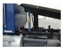
During maintenance or repairs, workers and mechanics must ensure blocking mechanisms are properly locked in place. If supports are not provided, proper blocking must be used with such equipment as jack stands or wood cribbing.
