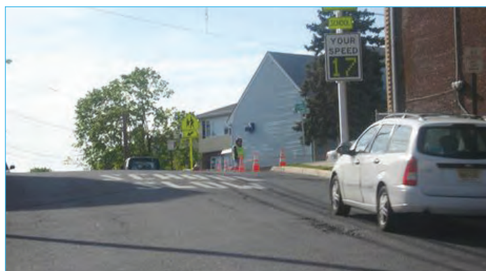
A radar sign was installed at this crossing station after an especially serious accident involving sun glare.
