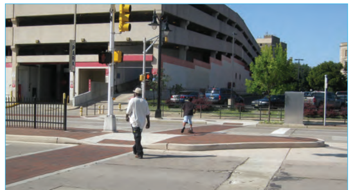
This pedestrian crossing has a center island, also known as a refuge that gives pedestrians a protected place to stand half way across the street.
